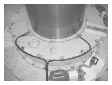
Many of BC Hydro's machines have permanent Eddy-current displacement probes installed to measure vibration. The displacement probes, with an output of 200 mV/mil, are used instead of accelerometers. The machines run around 300 rpm, speeds that are not very effective for accelerometers.
